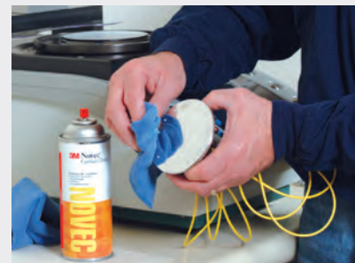
Wiping connectors in fixture with cloth and Novec Contact Cleaner.
