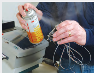
Applying contact cleaner to fixture with connectors.
