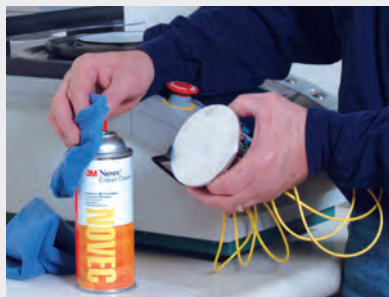
Applying contact cleaner to cloth.
